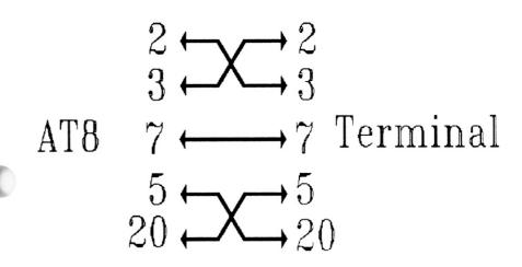
Figure 5.4: Cross over cable to DCE
