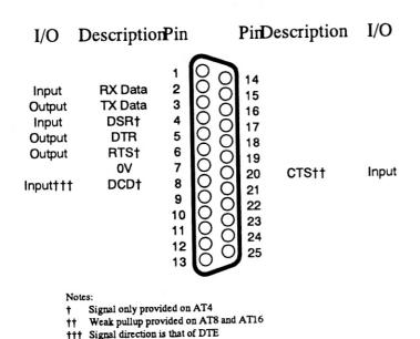
Figure 5.1: 25 Way Connector Pinout
