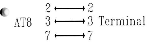
Figure 5.2: Software flow control Cable
